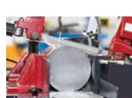
One of the most popular saw blades online, the 601 M42 bi-metal is designed to be an all-purpose, high-quality blade. We custom build each blade to have aggressive tooth geometry and a fatigue-resistant backer. And by setting the teeth alternately on the left and right side at regular intervals, we break up the regular tooth pattern to reduce noise, vibration, and chatter.
