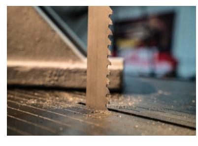
The 1001 CT is a Type 1 carbide-tipped band saw blade. The teeth have a beveled edge with a straight leading tooth, so it's wear resistant while cutting. It's also carbide tipped, which means it can handle tough materials that bi-metal blades cannot cut. These saw blades are commonly used to cut gates and risers, which is why it's referred to as a foundry carbide blade.
