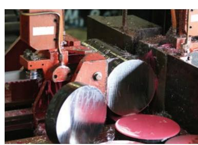
We craft these band saw blades with a new aggressive tooth geometry, making it perfect for cutting difficult-to-machine exotics and alloys. The tooth design, coupled with a triple-chip grind and positive rake angle creates smooth, fine-finish cuts.
