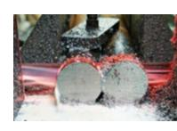
The 601 VTH Plus M42 bi-metal cuts through large solid sections of nickel or exotic-based alloys. Its variable tooth height and ground gullet give it extra chip carrying capacity, making it a unique blade in the sawing industry. We make the 601 VTH Plus extremely tough, and weld it for excellent heat and wear resistance. This blade is built to last.
