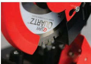
The Versatility of a Circular Chop Saw A circular chop saw uses a circular blade to cut wood, plastic, or metal. It's easy to operate and very portable making it a useful piece of equipment in most manufacturing operations as well as home shops. These saws accommodate a wide variety of blades for many different applications.
